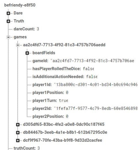
Figure 1. A snapshot of the Firebase Database web interface, showing the structure and value of variables in a JSON key-value format
